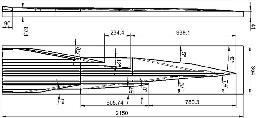
Fig. 2. An unfolded view of the wedge segment used for the rolling of the stepped shaft shown in Fig. 1 with marked wedge spreading angles  $\beta$ ; wedge diameter 800 mm.
