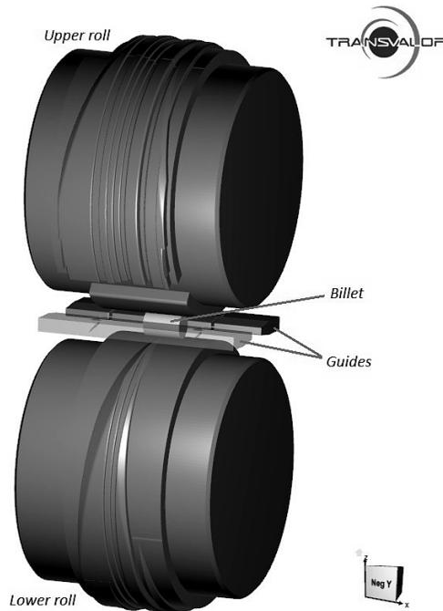
Fig. 3. Geometrical model of rolling a stepped shaft generated using Forge NxT 1.1 software.
