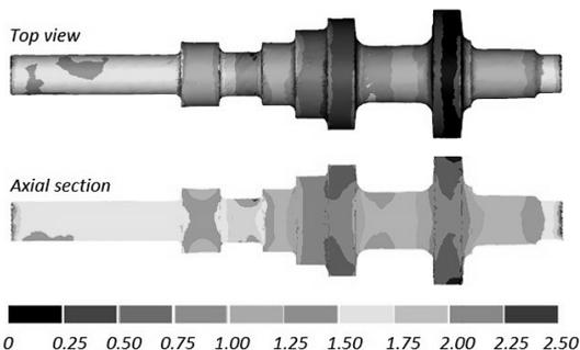
Fig. 8. Distribution of damage function, according to the Cockcroft–Latham criterion, determined using Forge NxT 1.1.
