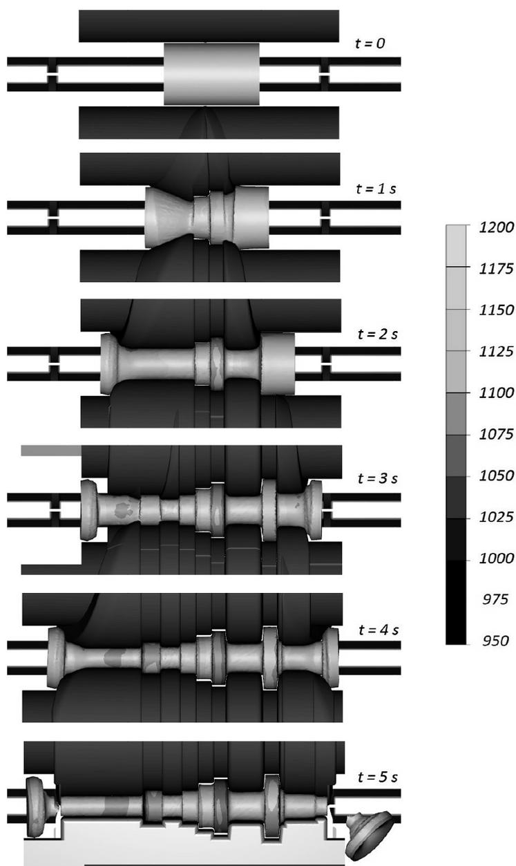
Fig. 5. A Forge NxT 1.1 simulation of the course of the rolling process for a stepped shaft, with colour-coded temperature distribution (in °C).
