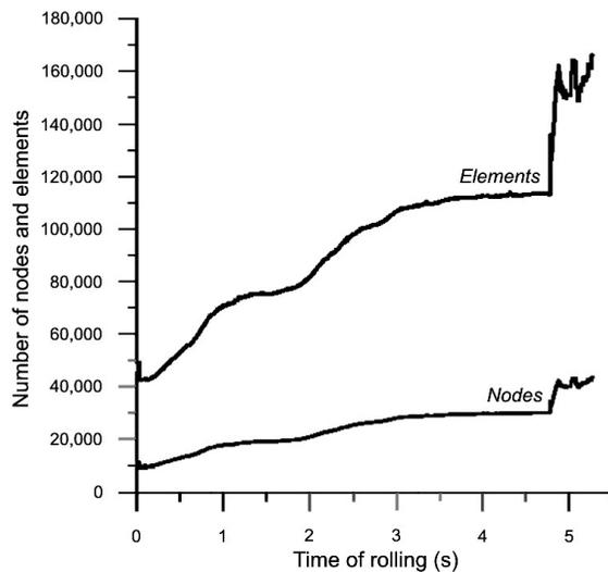
Fig. 4. Changes in the number of elements and nodes used in numerical calculations as a function of rolling time.
