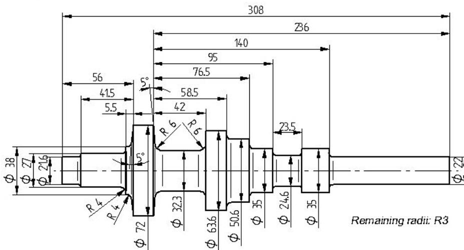
Fig. 1. Stepped shaft used in the numerical analysis.
