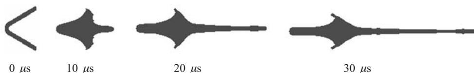
Fig. 8. Numerical simulation of the formation of PTFE jet at different times.
