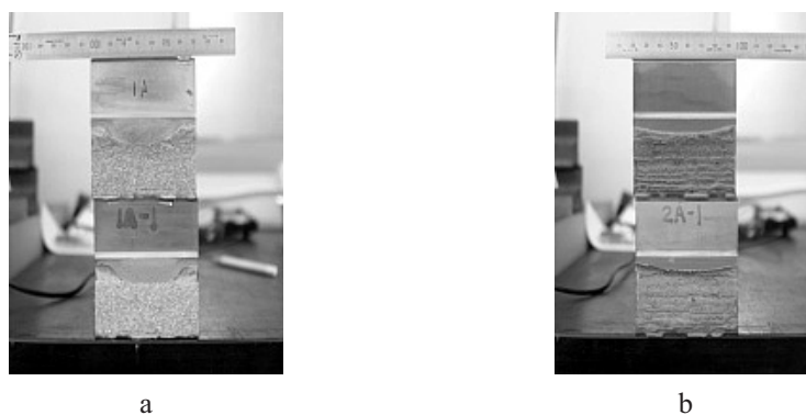
Fig. 5. Fractured EGW welded specimen after the CTOD test: surface notch (a) and through-thickness notch (b).
