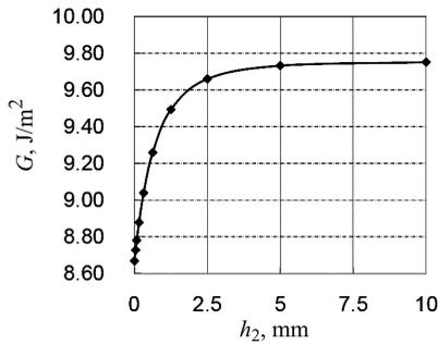
Fig. 4. Variation of strain energy release rate according to second layer thickness.
