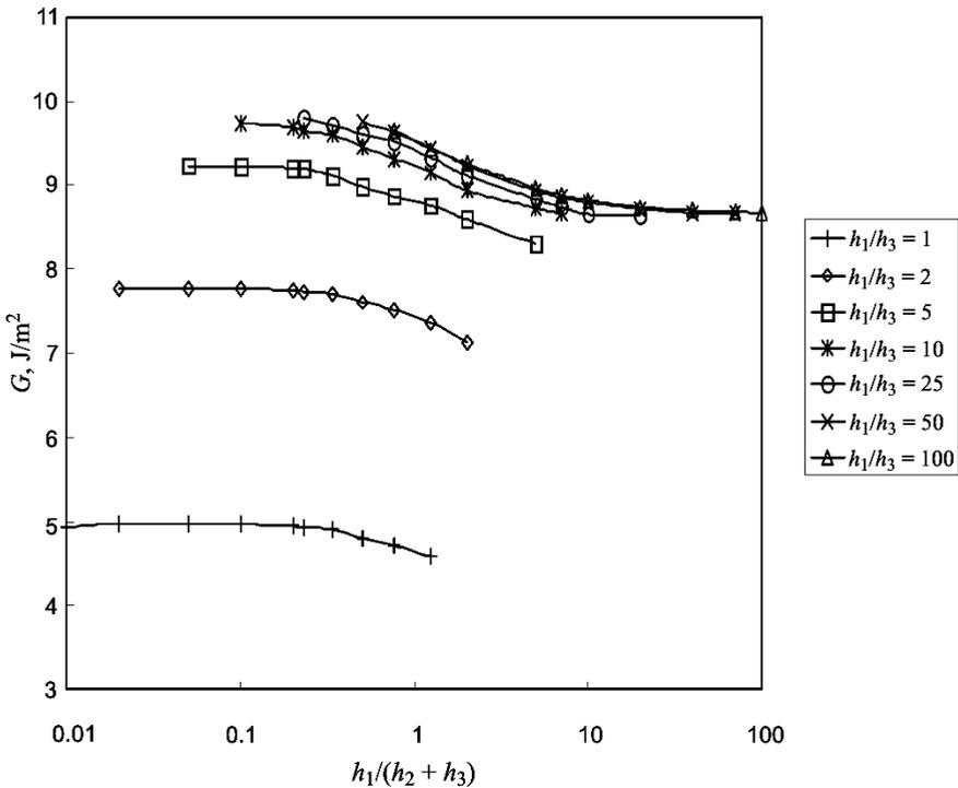
Fig. 5. Variation of strain energy release rate according to thickness ratios.
