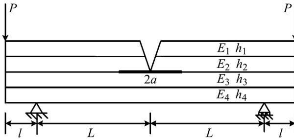
Fig. 1. Four-point bending test.
