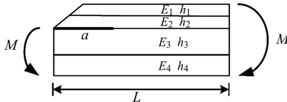
Fig. 2. Free-body diagram for the right half of four-point bending test specimen.
