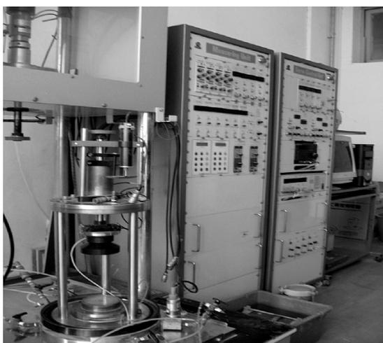
Fig. 3. Static-dynamic dual-purpose triaxial test apparatus.
