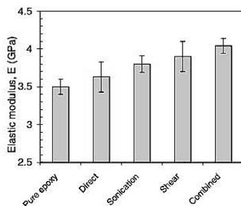
Fig. 1. Variation of elastic modulus of 1 wt.% EG/epoxy nanocomposites for different processing techniques.
