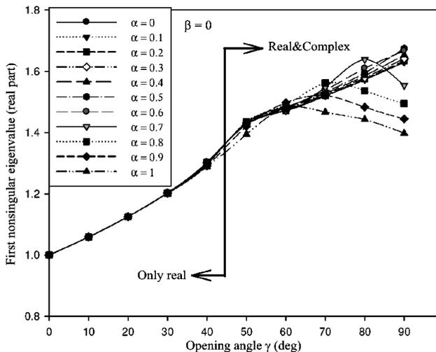
Fig. 7. Variation of real part of the first non-singular eigenvalue versus opening angle  $\gamma$  for  $\beta = 0$ .
