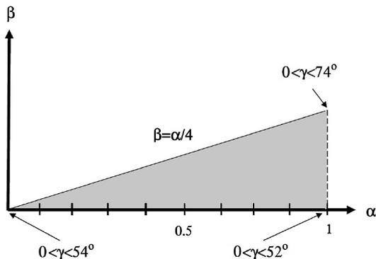
Fig. 11. Area with high order of singularity for the second singular eigenvalue in the range of  $0.5 < \lambda < 0.7$  limited by the maximum opening angles.
