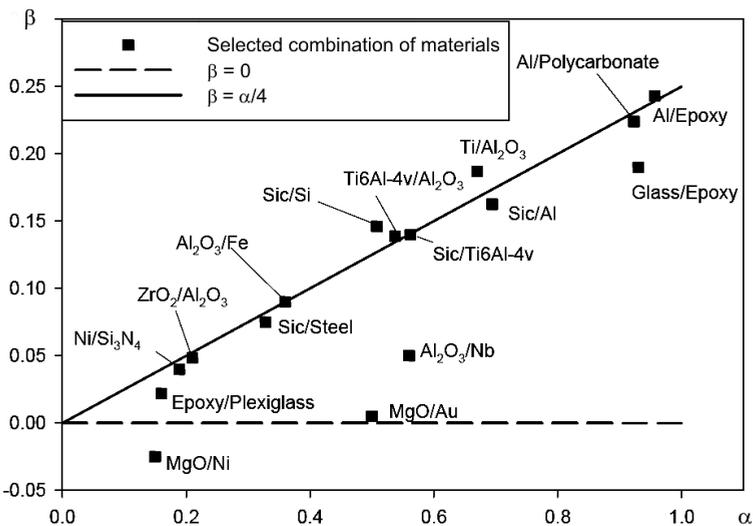
Fig. 2. Values of elastic mismatch parameters  $\alpha$  and  $\beta$  in plane strain condition for selected combination of materials [16].
