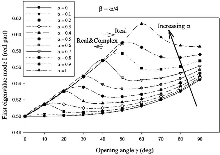
Fig. 4. Variation of real part of the first singular eigenvalue versus opening angle  $\gamma$  for  $\beta = \alpha/4$ .
