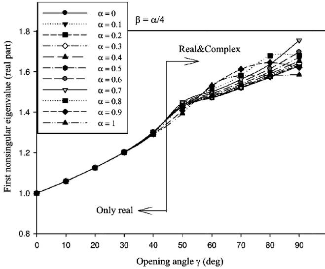
Fig. 8. Variation of real part of the first non-singular eigenvalue versus opening angle  $\gamma$  for  $\beta = \alpha/4$ .
