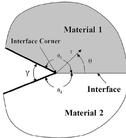
Fig. 1. General configuration of a bimaterial notch.
