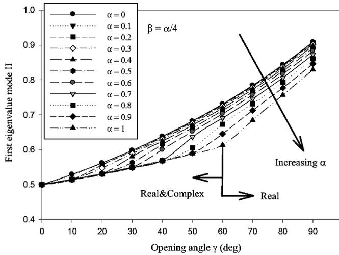
Fig. 6. Variation of real part of the second singular eigenvalue versus opening angle  $\gamma$  for  $\beta = \alpha/4$ .
