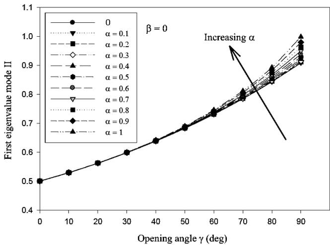
Fig. 5. Variation of second singular eigenvalue versus opening angle  $\gamma$  for  $\beta = 0$ .
