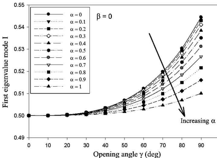
Fig. 3. Variation of first singular eigenvalue versus opening angle  $\gamma$  for  $\beta = 0$ .
