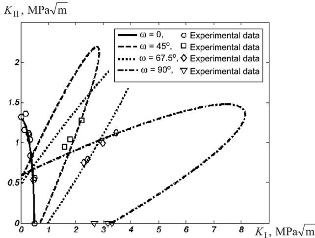
Fig. 9. Presented criterion for different crack orientation in comparison with experimental data [15] for Scots pine wood.
