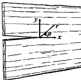
Fig. 1. Crack tip coordinate system used in the analysis of cracked wooden specimens.
