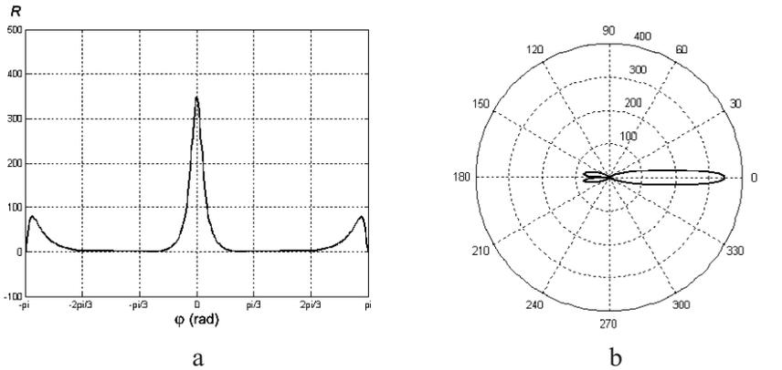
Fig. 3. Distribution of  $R$ -function in crack tip vicinity in Cartesian (a) and polar (b) coordinates for  $K_I = K_{Ic}$  and  $\theta = 0$ .
