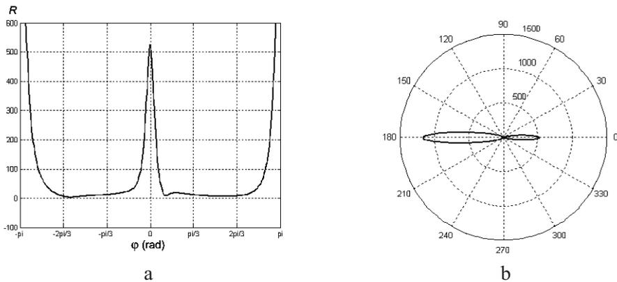
Fig. 4. Distribution of  $R$ -function in crack tip vicinity in Cartesian (a) and polar (b) coordinates for  $K_I = 0.4 \text{ MPa}\sqrt{\text{m}}$ ,  $K_{II} = 1.0 \text{ MPa}\sqrt{\text{m}}$ , and  $\theta = 0$ .
