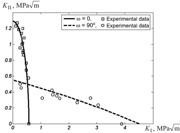
Fig. 8. Presented criterion for different crack orientation in comparison with experimental data [9] for Norway spruce wood.
