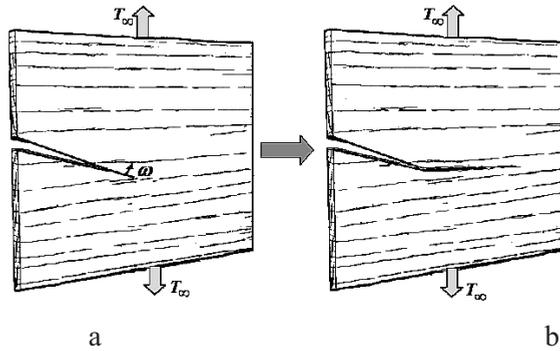
Fig. 7. Wood specimen with arbitrary orientation initial notch (a); kinking in an arbitrary crack orientation (b).
