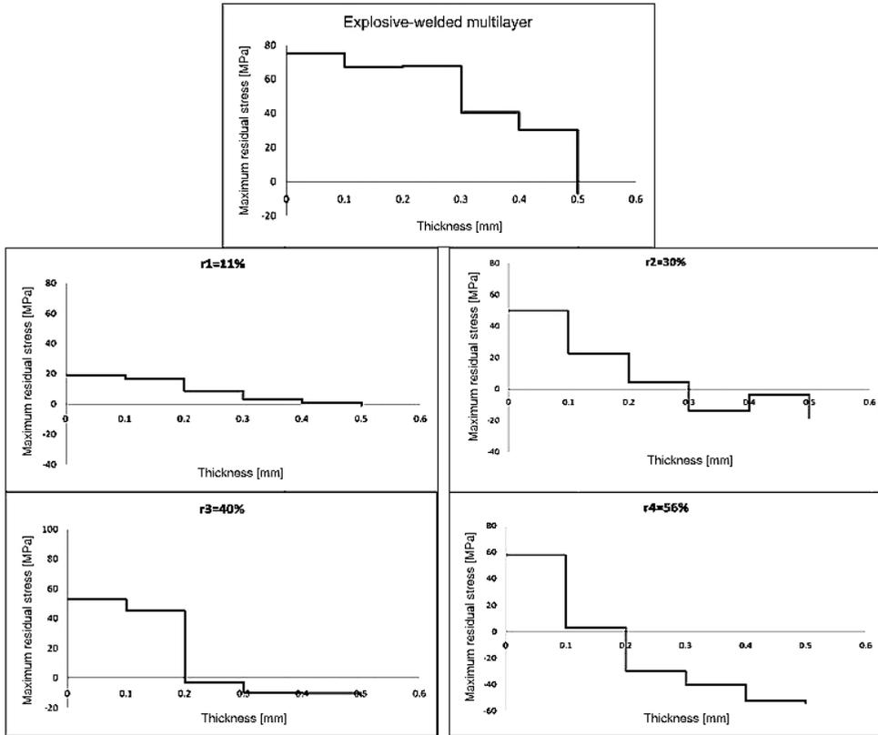
Fig. 4. Through-depth residual stress in explosive-welded and cold-rolled multilayers.
