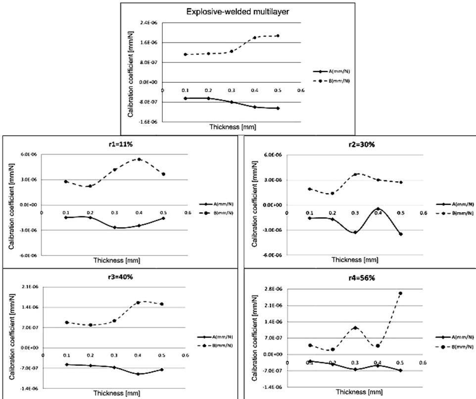
Fig. 3. Through-depth calibration coefficients in explosive-welded and cold-rolled multilayers.
