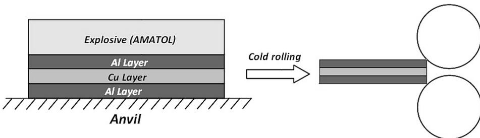
Fig. 2. Schematic view of parallel arrangement of explosive welding and cold rolling process.
