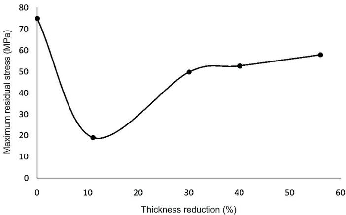
Fig. 5. Thickness reduction influence on surface residual stress.
