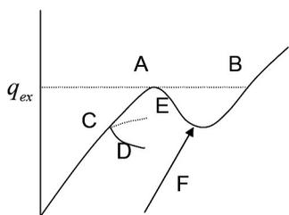
Fig. 3. Pressure–deflection curve of clamped shallow spherical shells.
