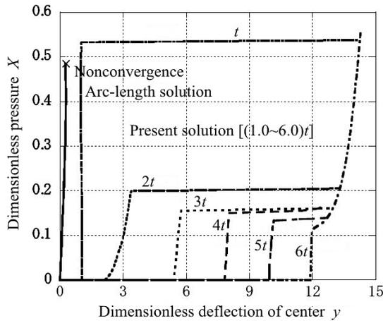
Fig. 10. Calculated critical snap-through arc-length solution results for  $\lambda = 6.5$  by the proposed procedure  $[(1.0-6.0)t]$  and arc-length solutions (nonconvergence) for clamped shallow spherical shells.
