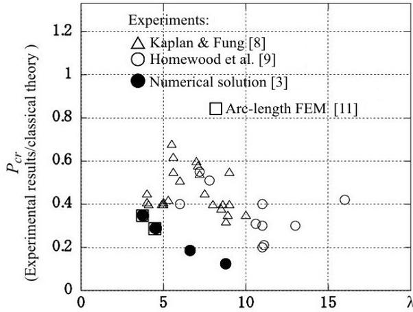
Fig. 4. Calculated lowest buckling pressure for an axisymmetric mode by Thurston and the arc-length solution with the experimental results.
