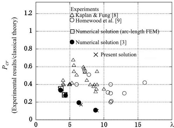
Fig. 11. Calculated lowest buckling of solutions, and arc-length proposed method and experimental results.
