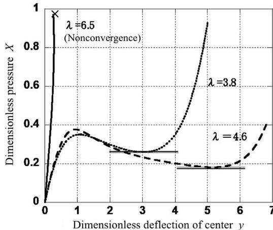
Fig. 5. Calculated critical snap-through arc-length solution results for clamped shallow spherical shells.
