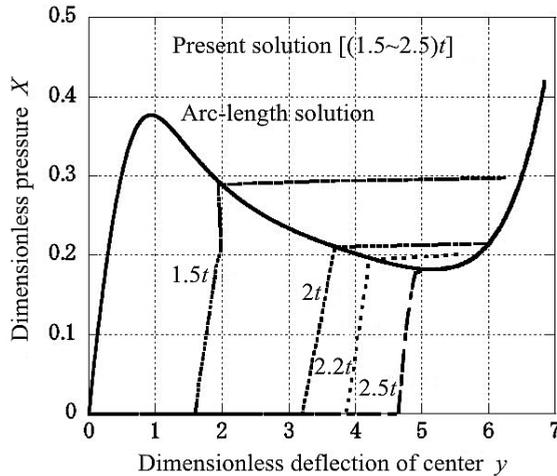
Fig. 9. Calculated critical snap-through arc-length solution results for  $\lambda = 4.6$  by the proposed procedure  $[(1.5-2.5)t]$  and the arc-length solution for clamped shallow spherical shells.
