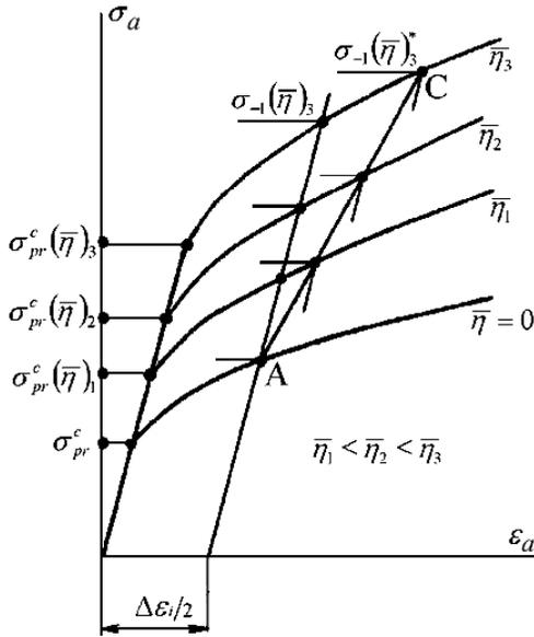
Fig. 6. Cyclic stress–strain diagrams for metals taking into account the stress gradient effect.
