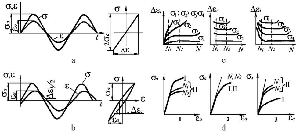
Fig. 1. Stresses and strains under high-cycle loading.
