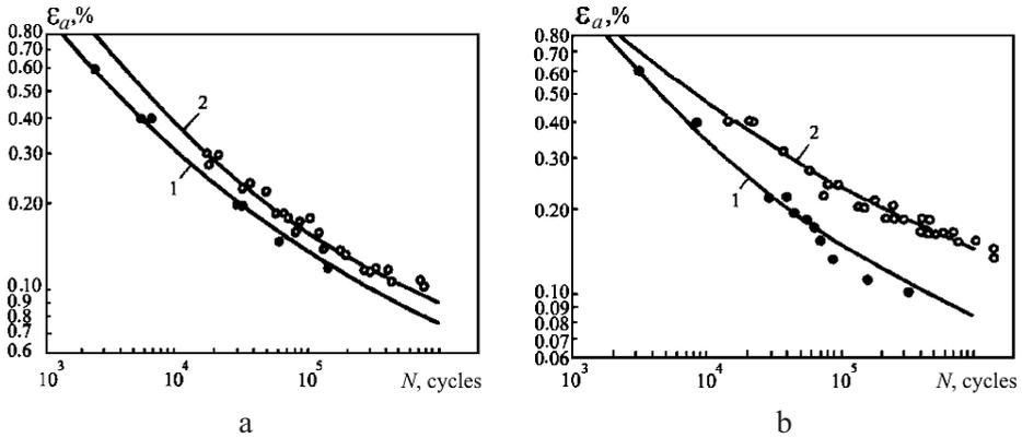
Fig. 4.  $\epsilon_a$  vs  $N$  relations under symmetrical tension for coarse-grained (a) and fine-grained (b) steels: (1) smooth specimens, (2) specimens with stress concentrators  $K_t = 1.54$  and  $2.57$ ).
