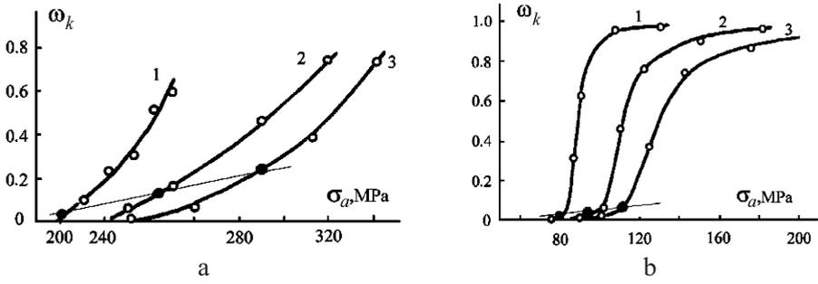
Fig. 3.  $\omega_k$  vs  $\sigma_a$  relations under axial loading and in bending: (a) low-carbon steel, (b) copper.
