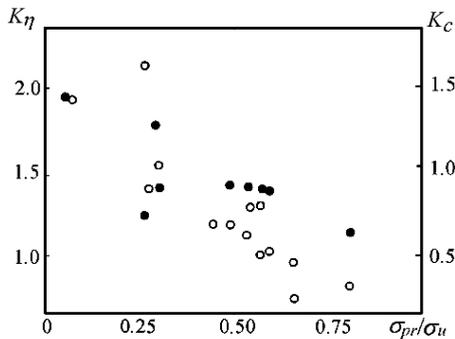
Fig. 7. Variation of  $K_\eta$  (●) and  $K_C$  (○) values depending on the  $\sigma_{pr}/\sigma_u$  ratio.
