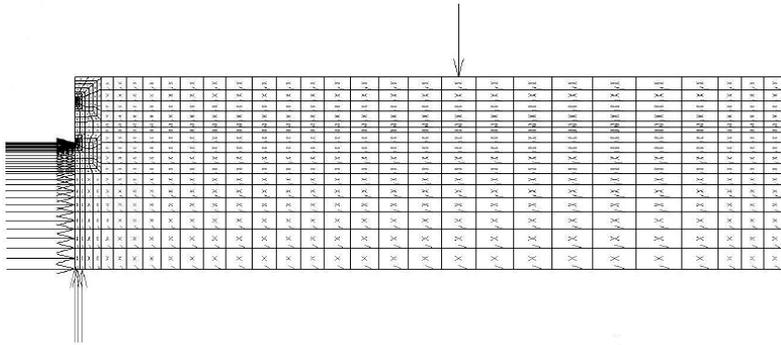
Fig. 1. Mesh of the large-scale Charpy-like 3PB specimen.
