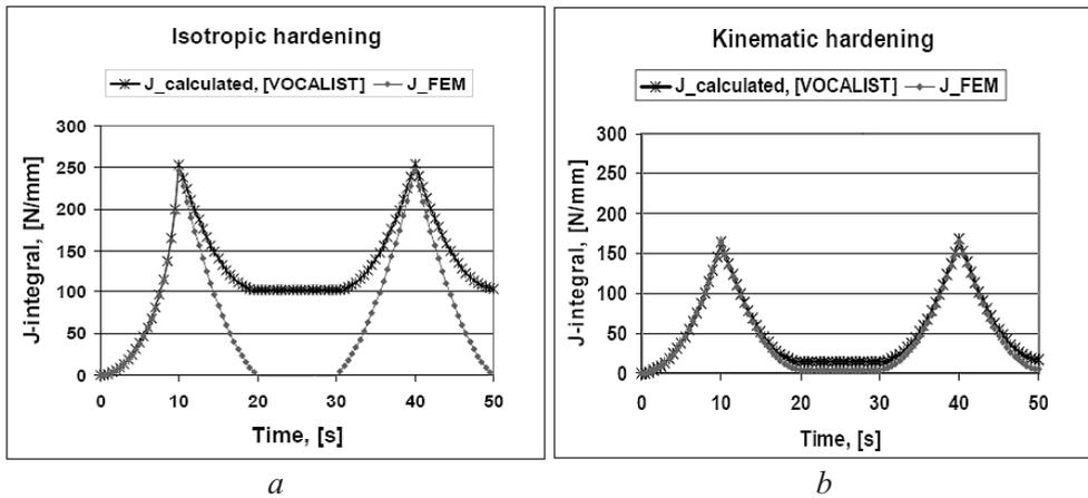
Fig. 5.  $J$ -integral curves under WPS condition in case of different hardening laws.
