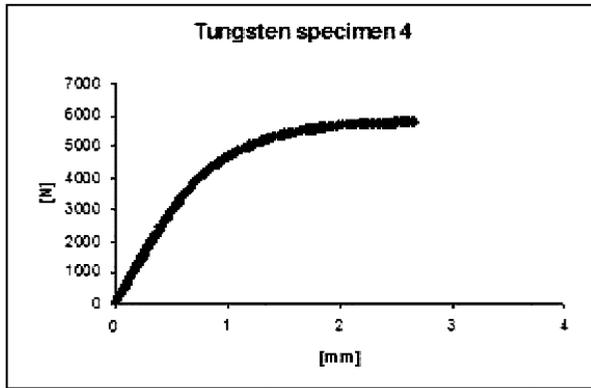
Fig. 5. Load-deflection curve from three-point bending test of irradiated tungsten bars.
