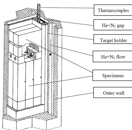
Fig. 3. Cross section of the BAGIRA irradiation rig.
