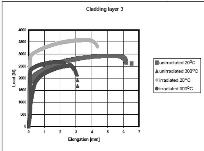
Fig. 4. Tensile results for RPV cladding.
