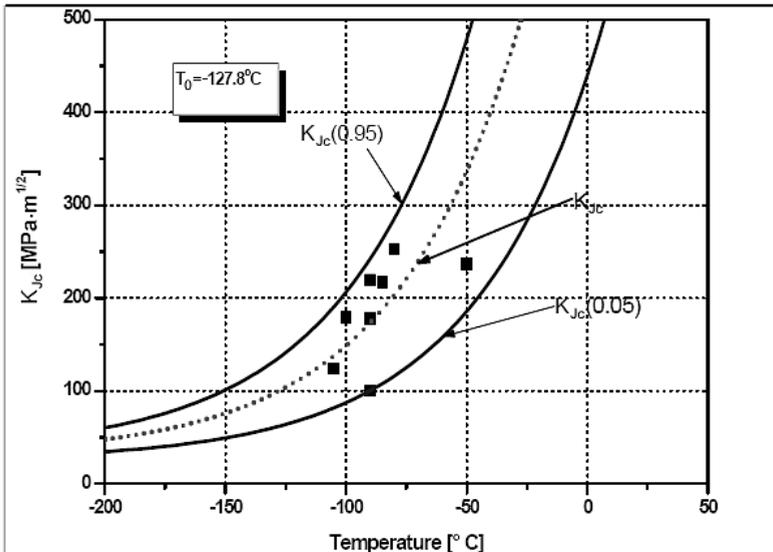
Fig. 6. Master Curve toughness testing results for 9% Cr steel.
