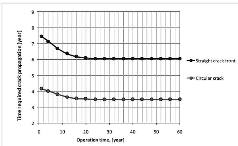
Fig. 4. Time required to reach an allowable stress corrosion crack size in a RVI component.
