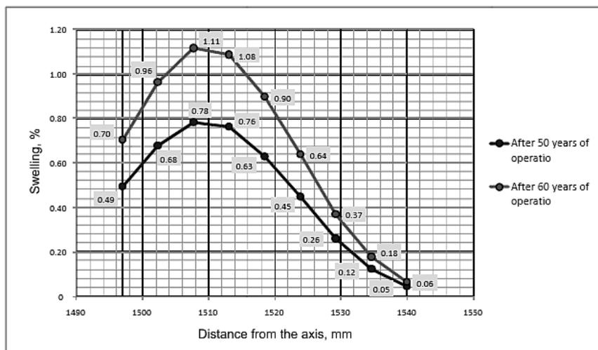
Fig. 5. Swelling effect in the basket wall after 50–60 years' operation.
