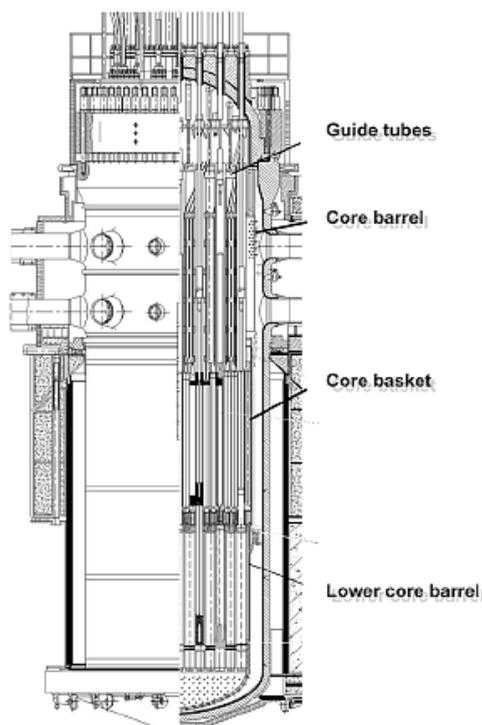
Fig. 1. Scheme of WWER 440 reactor pressure vessels and internals.
