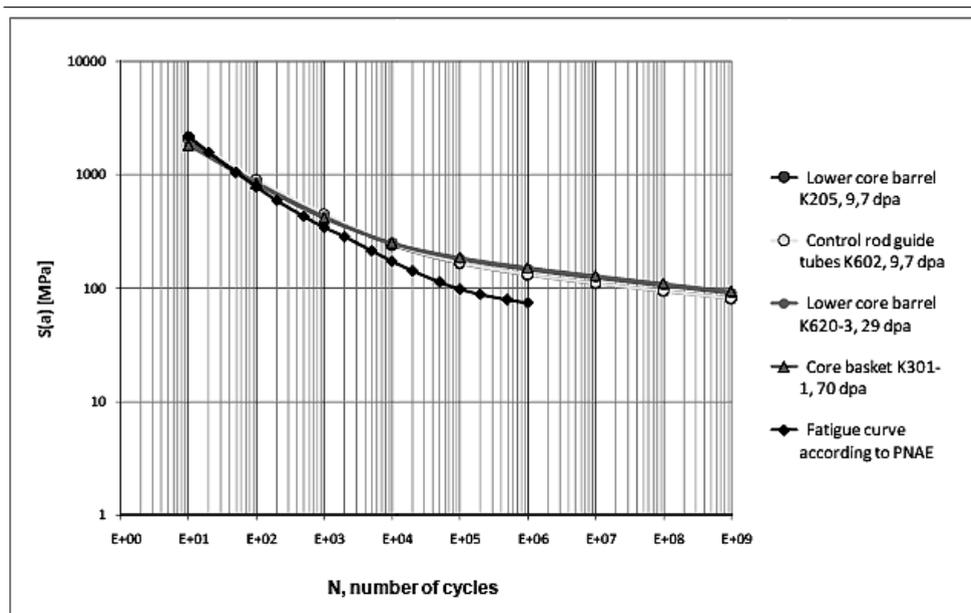
Fig. 3. Fatigue curves corresponding to 60 years' operation time ( $r = 0$ ).
